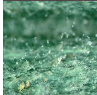
Fig. 5: Mould on test specimen 10 (H40), 40-fold enlargement.
