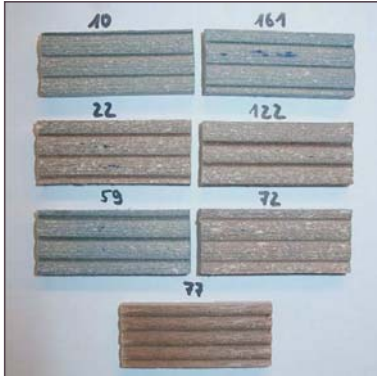
Fig. 3: Selected test specimens after the mould test: no vegetation macroscopically detectable.
