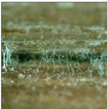
Fig. 9: Mould on test specimen 77 (Bangkirai), 50-fold enlargement.
