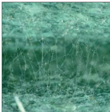
Fig. 7: Mould on test specimen 59 (H40), 40-fold enlargement.
