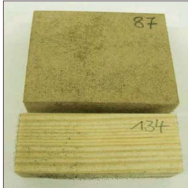
Fig. 4: Reference test specimen after mould test: vegetation clearly detectable (top: MDF, bottom: pine splint).
